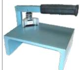
A sturdy rounder with interchangeable blades. Suitable for 1mm metal and 1½mm flexible plastics.
