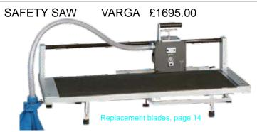
Traditional construction safety saw for cutting most types of material including flexible and rigid laminates, brass, foamex, wood and card. Maximum cut length 620mm and up to 6.3mm thick. Uses 350 watt, 15000rpm motor and 36 tooth carbide blade.
